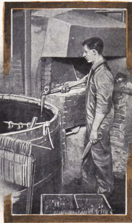
Hardening the Wiss Shear blade
